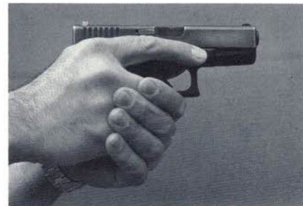
Close-up of hand and finger position on pistol. Trigger finger should be braced against receiver (or on front edge of trigger guard, provided trigger guard is not overly enlarged) to reduce possibility that finger will slip into trigger guard if officer's hand contracts involuntarily.
