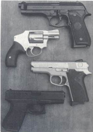
So-called "Double Action Only" handguns at least eliminate the possibility of an officer manually cocking his handgun. However, while their longer, heavier trigger pulls may reduce the likelihood of unintentional discharge, they do not eliminate it, and author feels finger should still remain outside trigger guard until the decision to fire has been made and the gun is raised to center mass. From top to bottom: Beretta Model 92D-P, S&W Model 642 Airweight Centennial (shown with Precision Gun Specialties Hideout grips), S&W Model 3953, and Glock 23 with "New York trigger."
